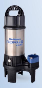
The CRXP model utilizes the same proven construction and components as the successful Norus series with the addition of an all new, high efficiency, single vane impeller. This unique impeller design produces higher flow rates than the standard Norus vortex impeller, yet still offers the same 1-1/4" solids handling capabilities. For the job that needs a little extra flow, the CRXP is the answer. High flow rates, high efficiency, high solids handling. Everything you expect from a ShinMaywa pump.
